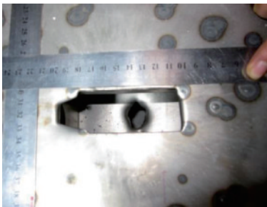
图8 顶板破口及破片冲击底板 Fig.8 Roof breaks and fragments impact the bottom plate
