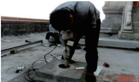
图7 倾斜仪现场测试 Fig.7 Field testing of the inclinometer
