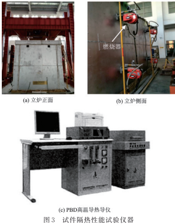
Fig.3 Furnace for thermal conductivity test of plates
