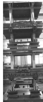
图42 两个大位移摩擦摆支座共同滑动呈第一振型 Fig.42 Vibration shape of two SLDRFPBs as first mode
