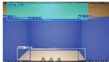
图6 通过实例分割深度学习模型识别的建筑组件 Fig.6 Building components identified by instance segmentation deep learning model
